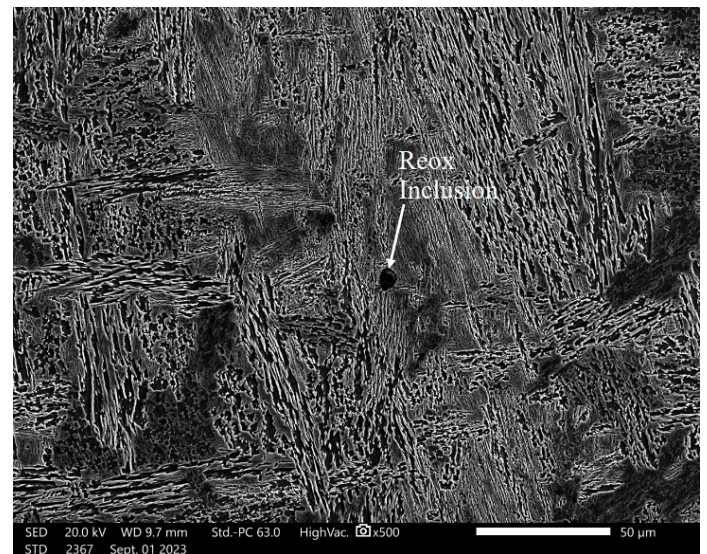
Figure 7. Typical microstructure of as-cast QP1.
